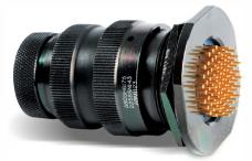
This British Standard version offers additional design advantages to the MIL-DTL-26482 Series 1 connector type. An economic, lightweight solution for use in a broad range of military, industrial and commercial applications. These connectors feature 3 pin bayonet coupling or an alternative "push-pull" version in shell sizes 10 and 12 for guick release applications.
