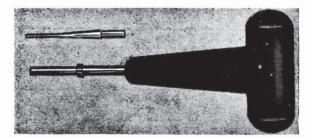
Each field service insertion tool has a coloured sleeve to provide easy identification of the correct size.
