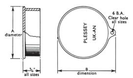
The range of transit caps for UK-AN connectors is designed to be a "push on" fit and to exclude dust, etc., when the connector is not in use. A 6BA clearance hole is provided on all sizes for use when a simple captive cover is required. Now supplied with all units when purchased.
