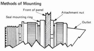
Mounting from the front when using cable fittings is limited to panels up to a maximum thickness of 0.135 inch for shell sizes 12s to 36, and 0.080 inch for shell size 10s. Panels of a greater thickness will prevent locking of the outlet nut.
