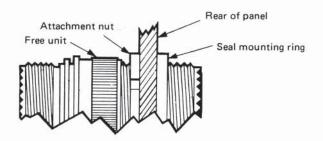
Mounting from the rear is limited to panels up to maximum thickness of 0.320 inch for 10s, 0.300 inch for 12s and 14s, 0.230 inch for 16 to 28, and 0.190 inch for shells 32 and 36. Panels of a greater thickness will prevent the free unit from mating to the correct extent.
