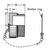
The anchorring is designed to screw on the thread at the rear of the Free Unit.
